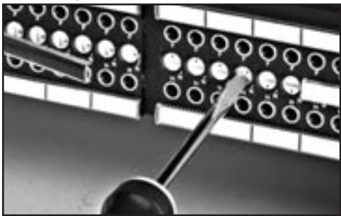
Easily Normal The Jacks By Rotating To "Full", "Non," Or "Half" Positions
